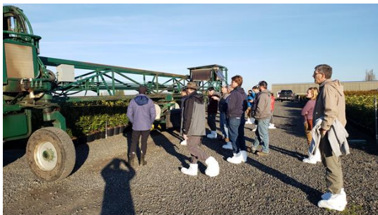
(A locally-engineered pruning machine (left) capable of capturing trimmings and self-disinfection (above) – Courtesy of C Hong)
